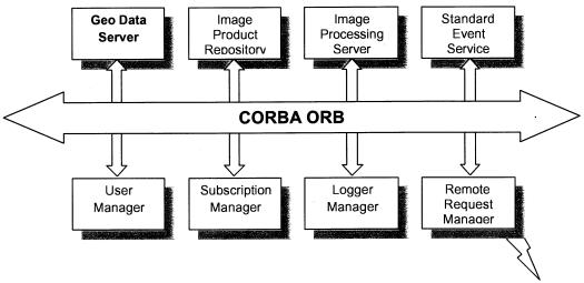
Fig. 3: Architecture of a RAMSES Core Server
