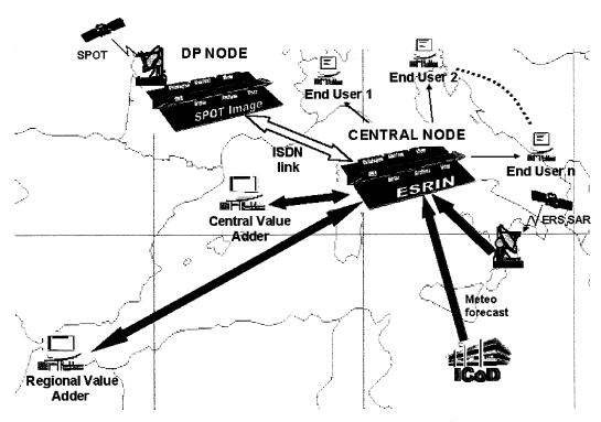
Fig. 2 Current RAMSES Topology: one central node + one data provider node.
