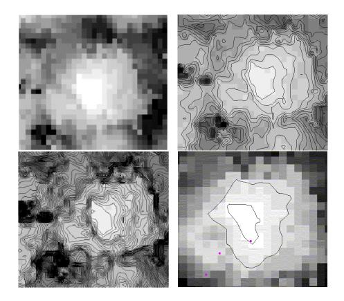
Figure 2: Upper left: Raster dataset showing one dominant Hornbeam (*Carpinus betulus*) crown in a broadleafed stand in the Rhine plain test-site. Upper right: Contour lines with a vertical distance of 100 cm. Lower left: Contour lines with a vertical distance of 25 cm. Lower right: Selected contour lines. Magenta dots: positions of stems.
