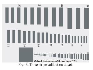
Images of the calibration target were recorded using the system and the ground resolved distance GRD was determined using the images.
