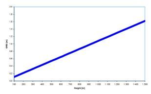
Graph 4. Ground resolved distance GRD of a 3CCD camera.
