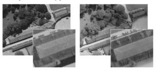
Figure 3: Comparing aerial film and digital image. Left is scanned film at a pixel size of 15  $\mu$ m (GSD of 15 cm); at right is the digital image with a GSD=17cm (from Leberl & Gruber, 2003).
