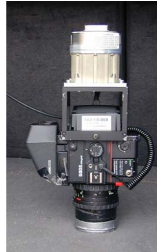
Figure 5: Litton 86-IMU mounted on Rollei db23
