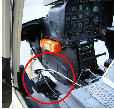
Figure 2. Integration of the equipment (IMU, VIS-Camera and Camera-Laptop) in a helicopter
