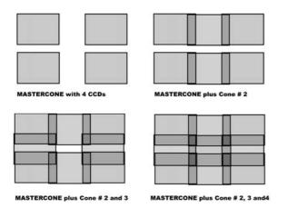
Fig. 2: The backplanes of four cones of the panchromatic channel produce a set of 9 sub-images. These get sequentially grouped in 3 steps, where 4 formats exist, which we denote as "layers". The master cone on the upper left with its 4 CCDs defines the geometry of the large format image.
