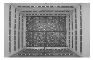
Fig. 3: Calibration test field in the basement of Vexcel's office building. The test field consists of 240 precisely surveyed control points.
