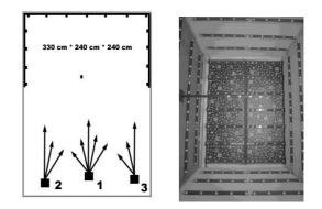
Fig. 4: Three Camera positions are established (left) and a set of 84 images is produced by rotating and tilting (right) the camera.
