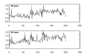
Fig. 6: Deviation of measured image coordinates of 200 target points in the set of 84 images in x-direction (top) and ydirection (bottom)
