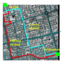
Figure 4. A part of the tested map and examples of routes
