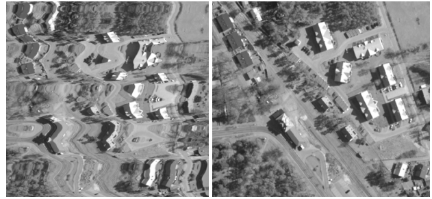
Figure 5. Robustness of geometric correction (left: raw data, right: rectified data)
