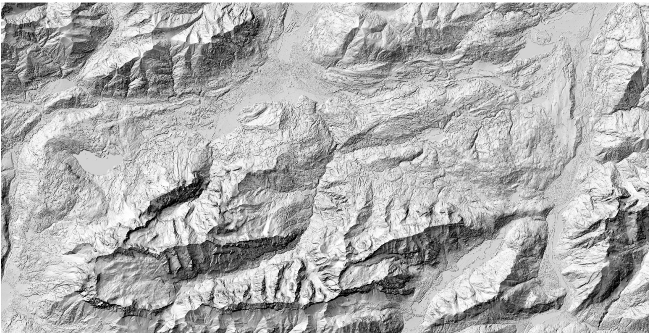
Figure 8. HRSC-AX ortho-image mosaic (15 cm/pixel) and DEM, shaded relief, (1m-grid) "Zugspitze" (Germany's highest mountain) and its vicinity (subset of approx. 500 km 2 ), Bavarian Alps.
