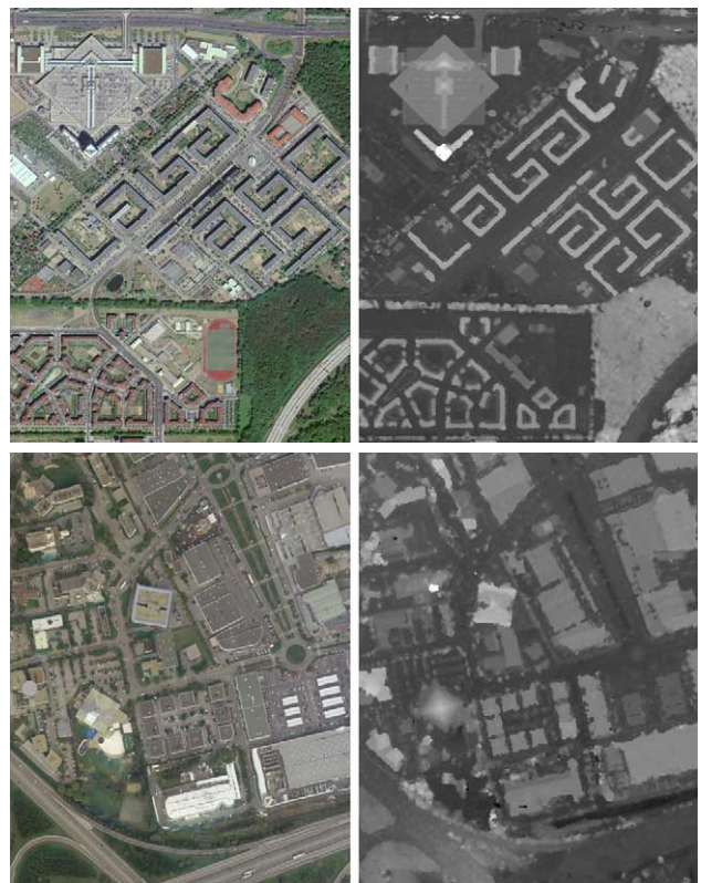
Figure 6. Subsets of ortho-images and digital surface models derived by DLR's processing system for multi-line scanners
