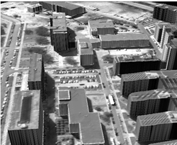
Figure 7. DSM Improvement of building shapes (Berlin, 2001, flight altitude 5,000m, subset Adlershof) top: perspective view using automatically derived HRSC DSM bottom: perspective view using vector enhanced DSM
