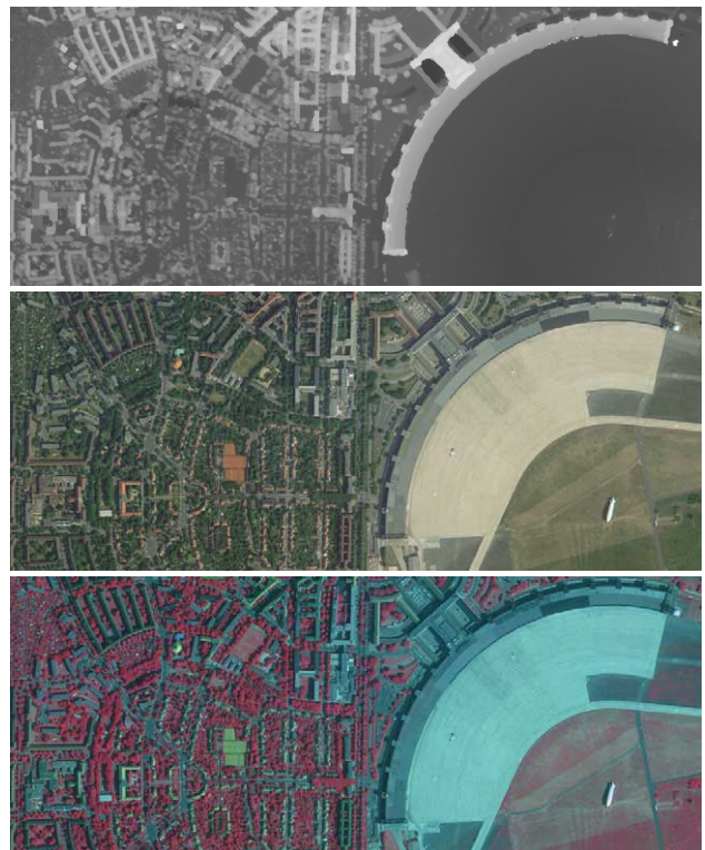
Figure 1. HRSC-AX standard products: 1m-digital surface model, true-color and CIR ortho-image mosaic (15cm/pixel) (Berlin 2003, flight altitude 4,400m, subset Tempelhof Airport)
