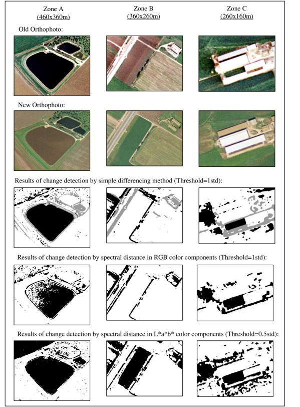
Figure 1: Examples of results of change detection experiences in three different zones and using three methods. Shown are the enhanced results by 5x5 majority filter.
