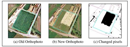
Figure 4: Example of changed pixel cluster which was detected as a part of large area object.
