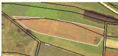
Figure 2. Problematic area, the black outlines represents cadastral plots, the white outline the real land use situation.
