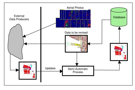
Figure 2. Dataflow for the revision process (after Hoejholt 2004)
