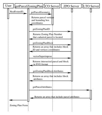
Figure 4. The UML sequence diagram of *getParcelZoningPlan* service
