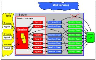
Figure 2. An example system configuration of C2IS [2].
