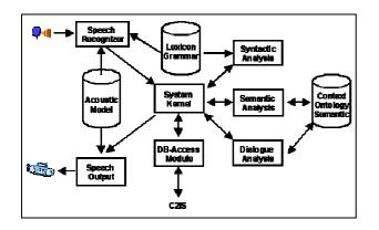
Figure 3. System configuration of HLT [2].
