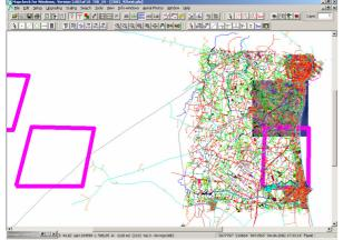
Figure 2. Shown is a block of update-data to be controlled together with the images, ready for photogrammetric transformation of vector data (X, Y, Z) in that area. Imagecoverage are shown with red lines. These are shown photogrammetrically, from the photocenter of the active photo
