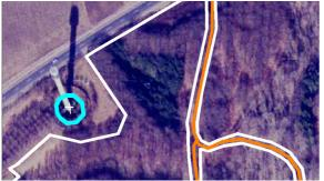
Figure 5. *Top:* Displaced objects caused by different object height specifications – by Vector Transformation (white trees in top and orange roads at bottom).
