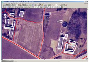
Figure 3. Example of Vector Transformation on raw image. The vector building shown close to silo has wrong Z value (0 m should be 72 m), and is displaced from its correct position by the road.
