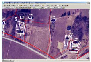
Figure 4. Same area as shown in fig. 3, from the polynomial rectified image (same fiducial and GCP's). Big displacements.
