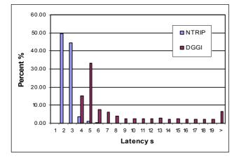
Figure 5. NTRIP-DGGI server comparison
