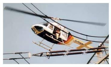
Helicopters are frequently used for the control of power lines, pipelines and other sensitive objects. Not only the control also first repairing from helicopters on the power line are undertaken, where exact navigation has to take place.
