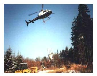
Figure 4: Helicopter for chalking forestry areas with the emitter under it
