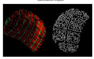
Figure 8. One mm contour lines of egg surface created from final point cloud after filtering gross errors
