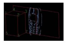
Figure 6. Point cloud of surface of cellphone after manual filtering of gross errors
