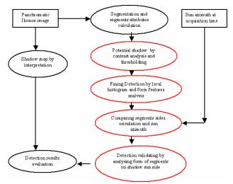
Figure 1: Diagram for the shadow detection
