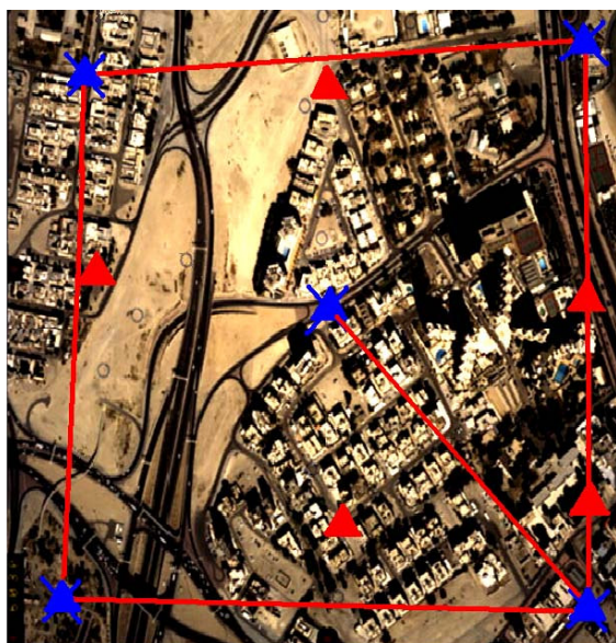
Figure 1. Aerial Photograph of an Urban City Center with Control (blue) and Check (red) Features Distribution
