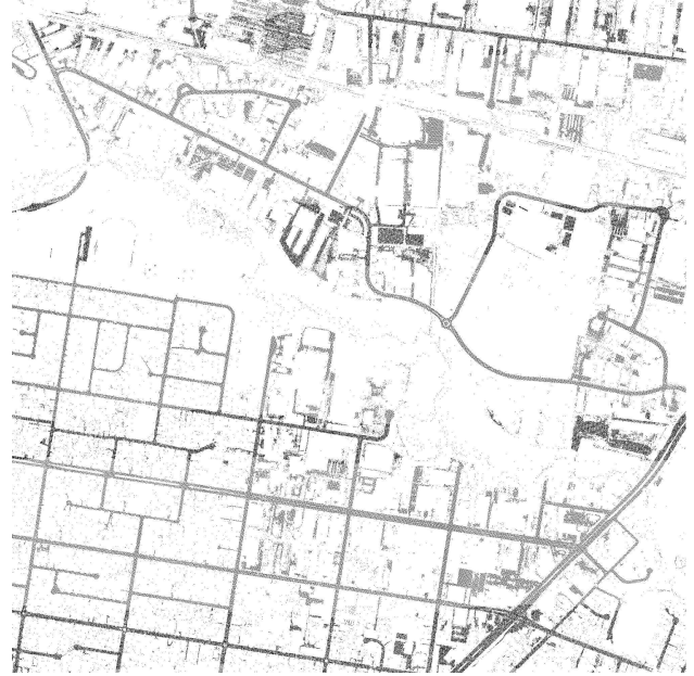
Figure 5: The road candidate points after intensity filtering.
