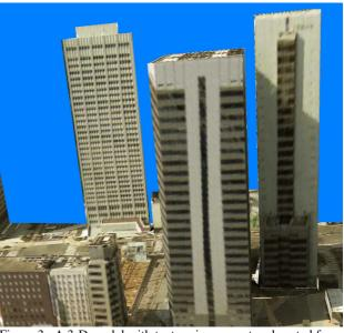
Figure 3. A 3-D model with texture images cut and pasted from aerial photos
