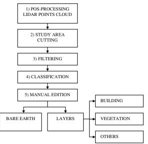
Figure 2. Flow chart of LIDAR data treatment.
