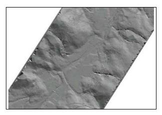
Figure 6. Part of DTM generated from integration of LIDAR points and aerophotogrammetric restitution elements.
