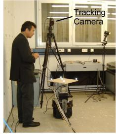
Figure 8. PLP-CAM robot and tracking camera
