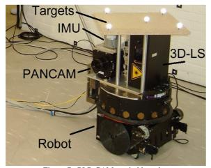
Figure 7. PLP-CAM carried by robot
