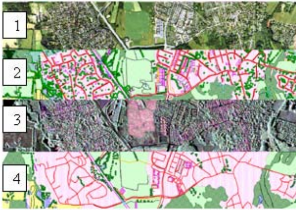
Figure 3: (1) - optical image (2) - Interpretation of optical image (3) - SAR-image (4) - Interpretation of SAR image
