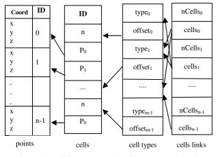
Figure 2. Implicit representation of geometry and topology
