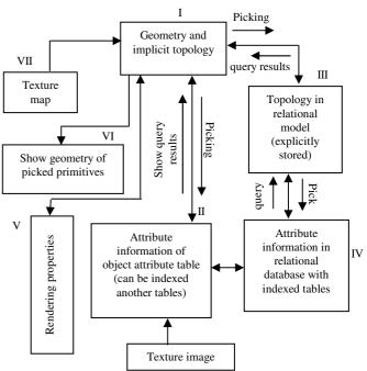
Figure 3. General representation of geometry and topology
