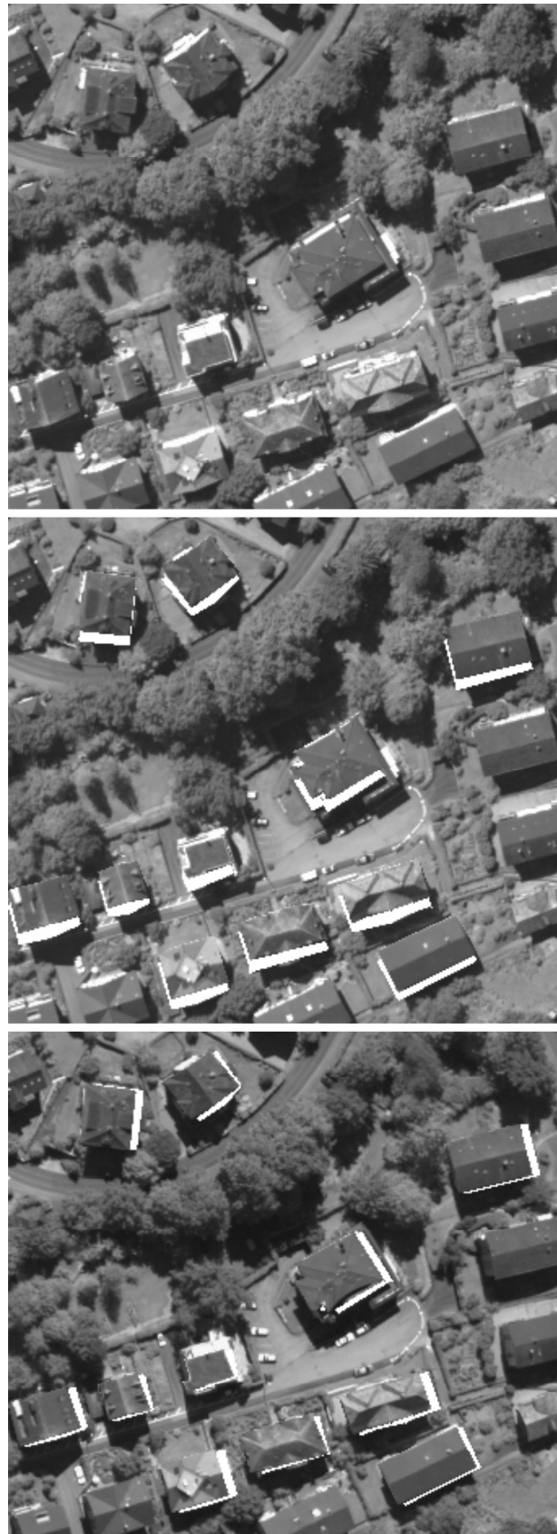
Figure 5. At the top, part of a residential area imaged by HRSC-AX in x-direction. In the middle, corrected image in y-direction, based on a dataset imaged in x-direction. Below, corrected image in x-direction, based on a x-directed overflowed dataset.
