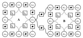
Figure 4: Internal representation of the two rectangles of figure 3 as a graph connecting unknowns by constraints. Unknowns are depicted as circles, constraints as boxes. The icons represent the "rectangular" and "point on line" constraints.
