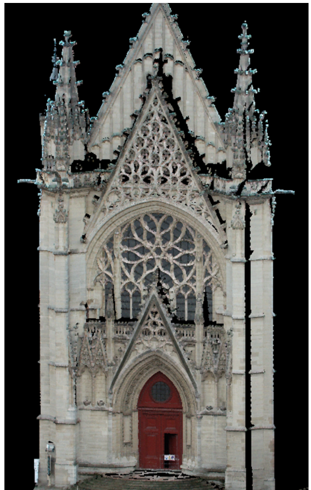
Figure 10: Results on the Vincennes castle chapel. Here, we show the point cloud, where each point has been assigned its image radiometry.
