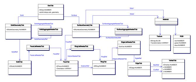
Figure 4. Object-relational database schema for the 3-D city model
