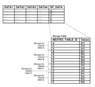
Figure 3: Example for a nested table, embedded in an object table. Each row of this object table corresponds to several rows in the nested table, representing a m:n-relation The figure is taken from (Oracle, 2002a).
