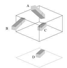
Figure 6. Example for an application of the query in Figure 5. The objects A, B and C interact with the bounding box and pass the filter, while D does not. The projections of A and C onto the x-/y-plane are inside the projection of the bounding box, thus both constitute the final result set. Note that only C is inside the bounding box.
