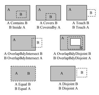
Figure 2: Topological relations differentiated by the function SDO\_GEOM.RELATE, which implements the 4-intersection model (Oracle, 2002b).
