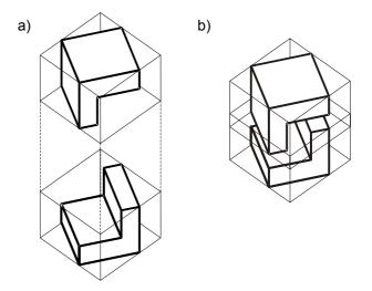
Figure 1: Approximation of geometries by minimal bounding boxes, yielding inexact results. In Figure a), both objects can be distinguished from each other, while in b), the two geometries do not touch each other, but their bounding boxes do so.
