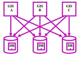
Figure 1 Interoperability Based on Direct Access to Databases
