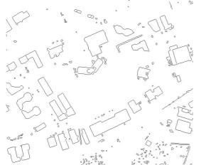
Figure 4: Delineation of buildings using Canny edge detector on the LIDAR elevation data
