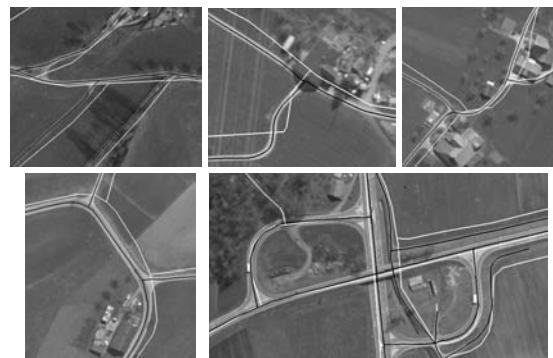
Fig. 2. Details of road extraction and junction generation with varying complexity in test sites in Switzerland. The extracted roads are shown in black lines and the VEC25 roads in white lines.
