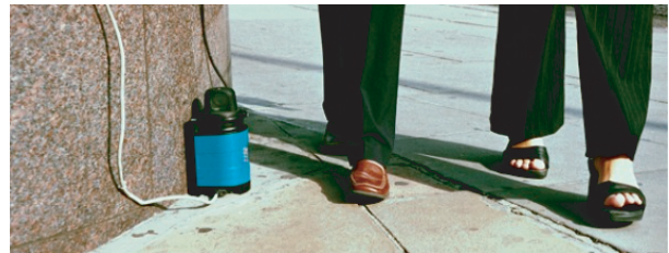
Figure 1: Pedestrian Measurement by using Laser Scanner
