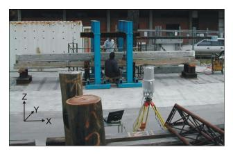
Figure 2. Concrete beam and the Riegl LMS-Z210.
