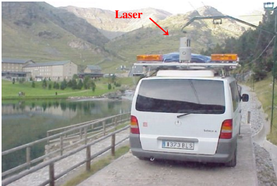
Figure 5: Terrestrial Laser integrated in the Geomöbil
