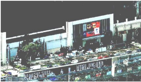
Figure 9: RGB laser points collected in a kinematic survey (laser looking to the right side of the van)
