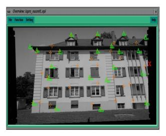
Figure 2.Measured Control Points for exterior orientation
