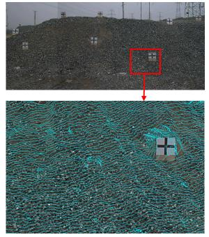
Fig. 5 PTSS has been used to measure stone pile. (a) Measurement scene (b) Contour
