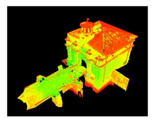
Figure 12. Final result of the global registration obtained with the Cloud Constrain Wizard
