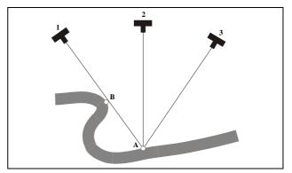
Figure 1. Due to small modeling, calibration and orientation errors, the texture of point B on image 1 may be assigned to A.
