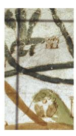
Figure 4. The gridline intersections were used as control information. Because the grid was lifted a few centimetres up from the map surface, the intersections appear to be a little bit different places on different images. The size of these pieces is about 2,0 cm x 3,5 cm and the same area can be seen in the upper right corner of the figure 3.
