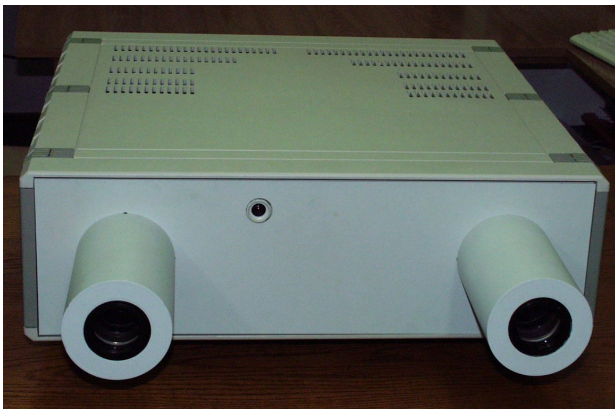
Fig. 3.3 The projection moire system [Zawieska, 2003]
