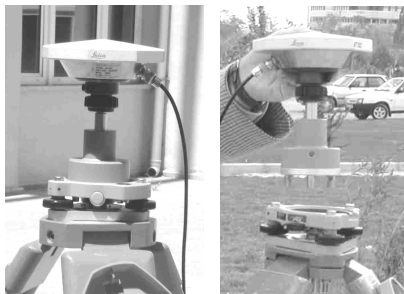
Figure 1: Removing GPS antenna from the levelled tribrach
