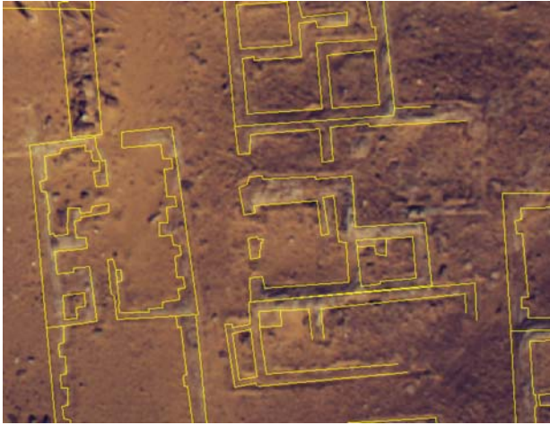
Figure 11. Superimposition of orthomosaic with vector drawing derived from topographical terrestrial survey (detail for a flat area near the Temenos ).
