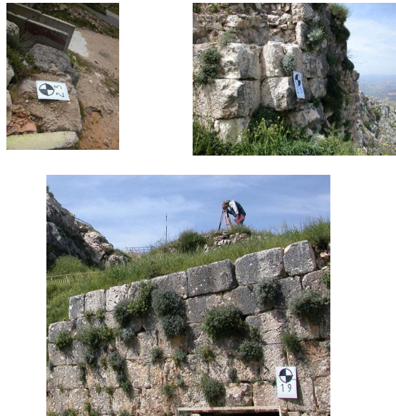
Figure 6. Examples of targets used for the control points
