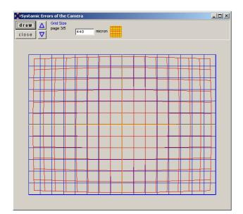
Figure 5. Distortion of wide-angle status (red: current distorted image, blue: ideal undistorted image)
