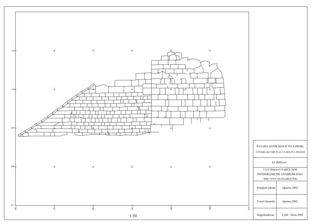
Figure 9. Evaluation result of a facade (original 1:50)
