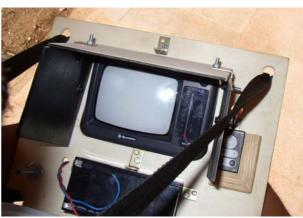
Figure 4. Ground control unit with monitor in the centre, remote controller on the right and battery for the monitor downside of the monitor
