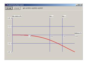
Figure 6. Radial distortion curve of wide-angle status
