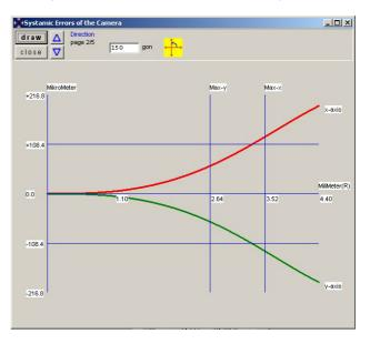
Figure 7. Total distortion curves along predefined directions (red: x-axis; green: y-axis)
