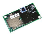
Figure 3. A sensor board that is equipped with a GPS receiver. (MTS420CA, Crossbow Inc.)
