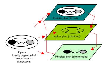
Figure 1. The three plans of a general system (adapted from Schwarz 1994)
