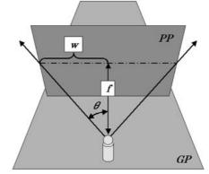
Figure 3-2. Relationship between focal length and field angle
