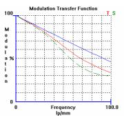
Figure 7. MTF measurement of the intercepting optical plate
